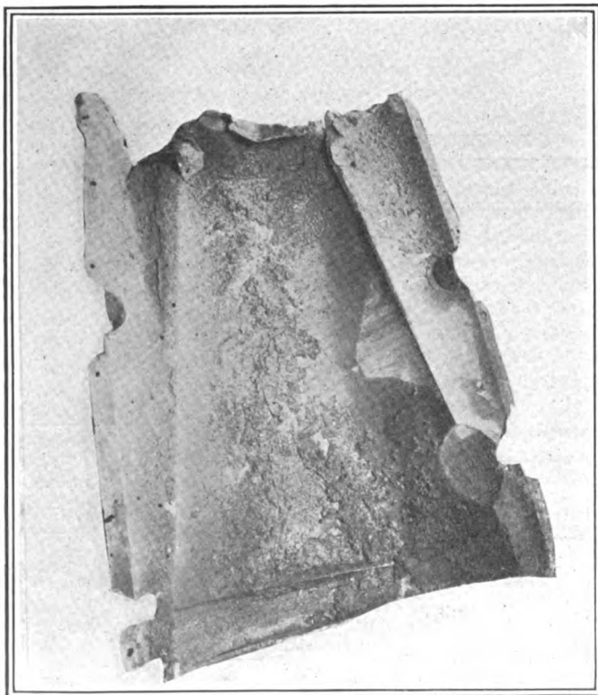
Fig. 1—Battered mudpan which was swung so low that it struck the road
